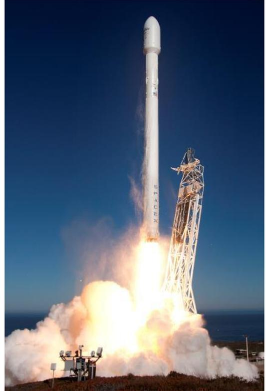
Three seconds before launch, the nine Merlin engines of the first stage ignite. The rocket computer commands the launch mount to release the vehicle for flight, and at T-0 Falcon 9 lifts off, putting out 1.3 million pounds of thrust.
