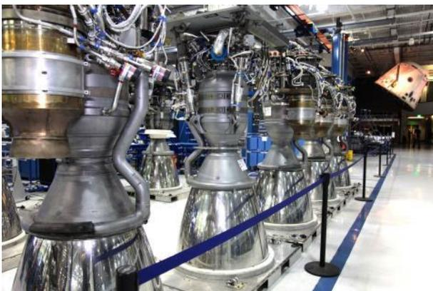
Falcon 9 is the only vehicle currently flying with engine out capability; Falcon 9 can lose up to two of its Merlin engines on the first stage and still complete its mission. The nine-engine architecture on the first stage is an improved version of the design employed by the Saturn I and Saturn V rockets of the Apollo program, which had flawless flight records in spite of engine losses.
