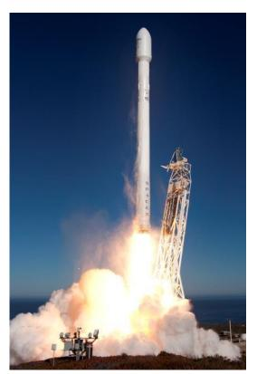
Three seconds before launch, the nine Merlin engines of the first stage ignite. The rocket computer commands the launch mount to release the vehicle for flight, and at T-0 Falcon 9 lifts off, putting out 1.3 million pounds of thrust.
