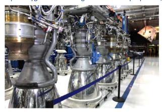
of thrust at liftoff, rising to 716 kilonewtons (147,000 pounds) as it climbs out of Earth's atmosphere. Merlin's thrust-to-weight ratio exceeds 150, making the Merlin the most efficient booster engine ever built, while still maintaining the structural and thermal safety margins needed to carry astronauts.
